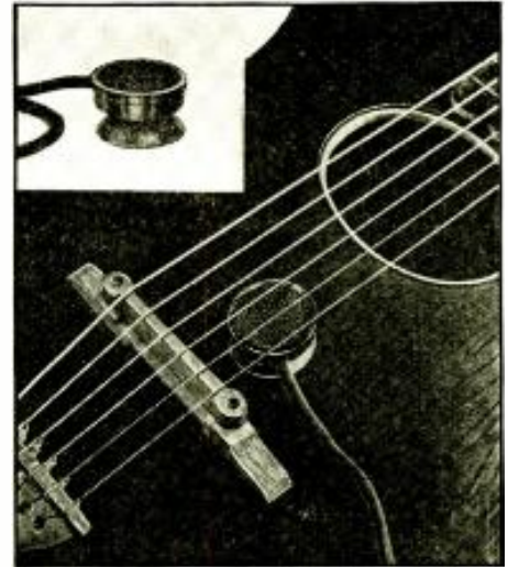
Fig. 1. An electronic pickup for converting musical instruments into electronic instruments. The "contact-type" microphone attaches to the instrument by means of a rubber suction cup (see inset).
